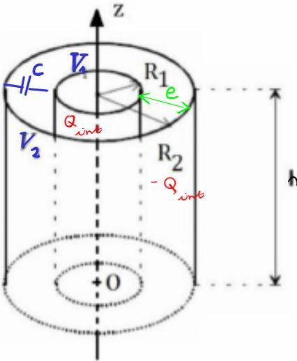
$$\Delta V = V_1 - V_2 = \frac{Q}{C}, \quad C?$$
